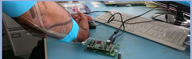
Lab demonstrator of MoniShirt sensing system.
